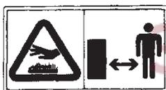
The muffler becomes very hot during operation and remains hot for a while after stopping the engine.
